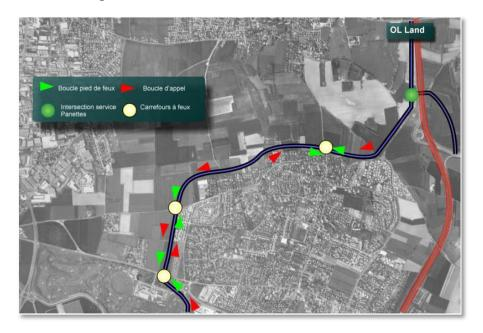
A dynamic simulation of the most strained intersection has been realized, to verify the shared road functioning, between vehicles and the high frequency of the bus circulation to bring spectators to the Stadium. This dynamic simulation should determine the degree of freedom for the priority system of bus lanes.
